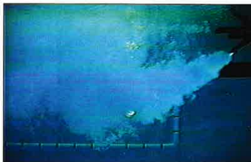
A 2-hp AIRE-O2 Aerator below the surface
